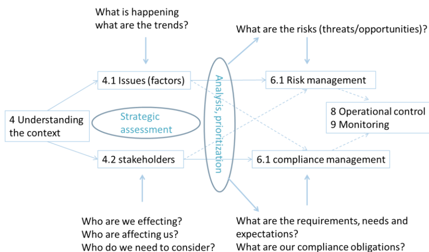
Figure 4 – HLS-structure presented as a horizontal process for context, analysis and control
